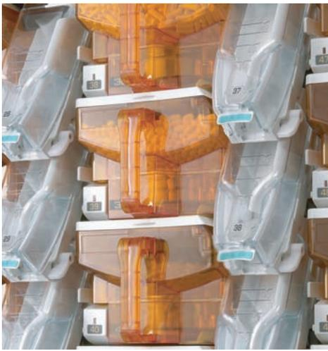
The EV-54 has a locking cassette system for added security and inventory control.
